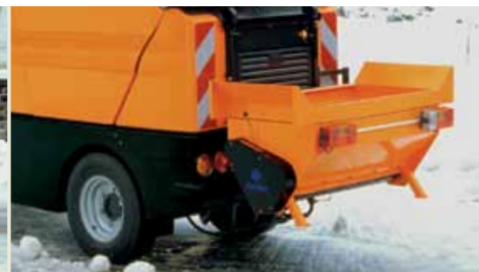
Snow brush and salt and sand spreader
