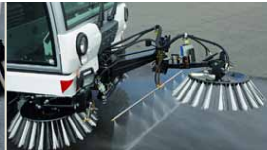
Street wash system
